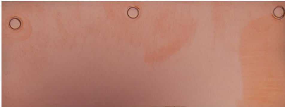
Figure 8. Copper analysis after 800 days in operation. Sample taken close to the end of the block.
