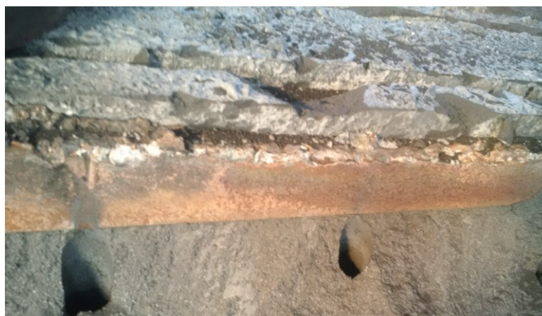
Figure 3. Aluminium deposited on bottom of copper bar.
