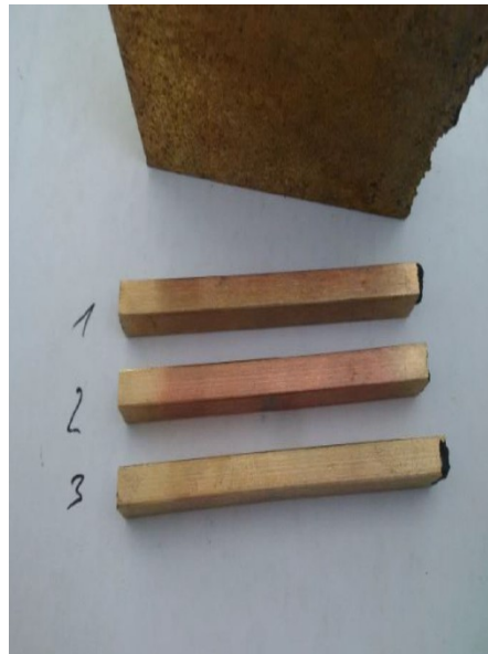
Figure 4. Cu bars samples with different extent of alloyed copper.
